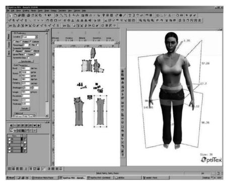
5.1 Control and positioning of 3D objects and adjusting cutting parts with parameters of prototype.
