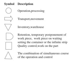
5.15 Display symbols that are used to map the flowchart process.
